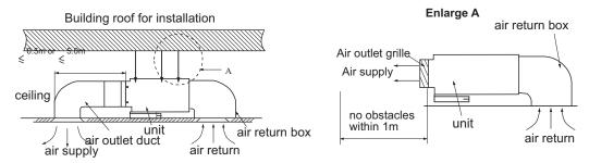
The distance between the duct air outlet and the air conditioner air outlet will depend on the actual duct length and the actual static pressure terminal:
