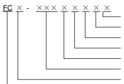
design serial number, A  $\sim$  Z applicable voltage, refer to below table air return type, refer to below table installation type, refer to below table external static pressure, refer to below table air flow (10 m³/h) appearance code, refer to below table fan coil
